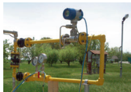
Mobile metering system with a flanged OPTISWIRL 4070 C
