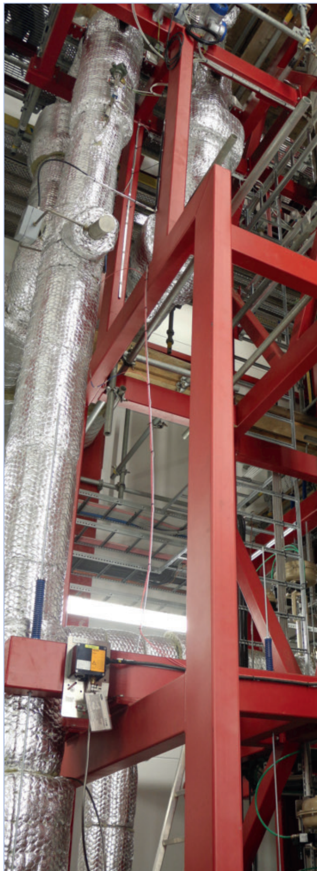
Ultrasonic flow measurement of a high temperature hydrogen/steam mixture
