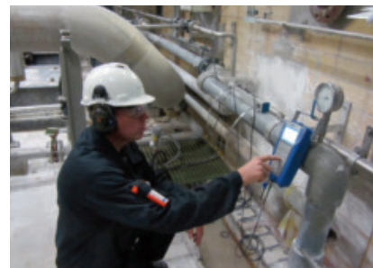
The OPTISONIC 6400 with mobile signal converter attached to a pipeline
