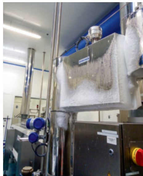
Mass flow measurement of liquid nitrogen for tunnel freezers with the OPTIMASS 6400 F
